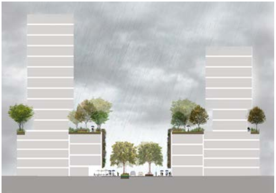
Figure 12. Typical secondary street section showing the design of blue corridors (image credit: Realm Studios)
