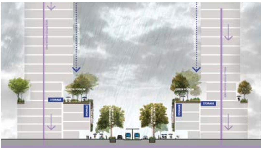
Figure 17. Podium scale building development highlighting opportunities for a third pipe to collect greywater for reuse and maximising horizontal areas for green infrastructure (image credit: Realm Studios)
