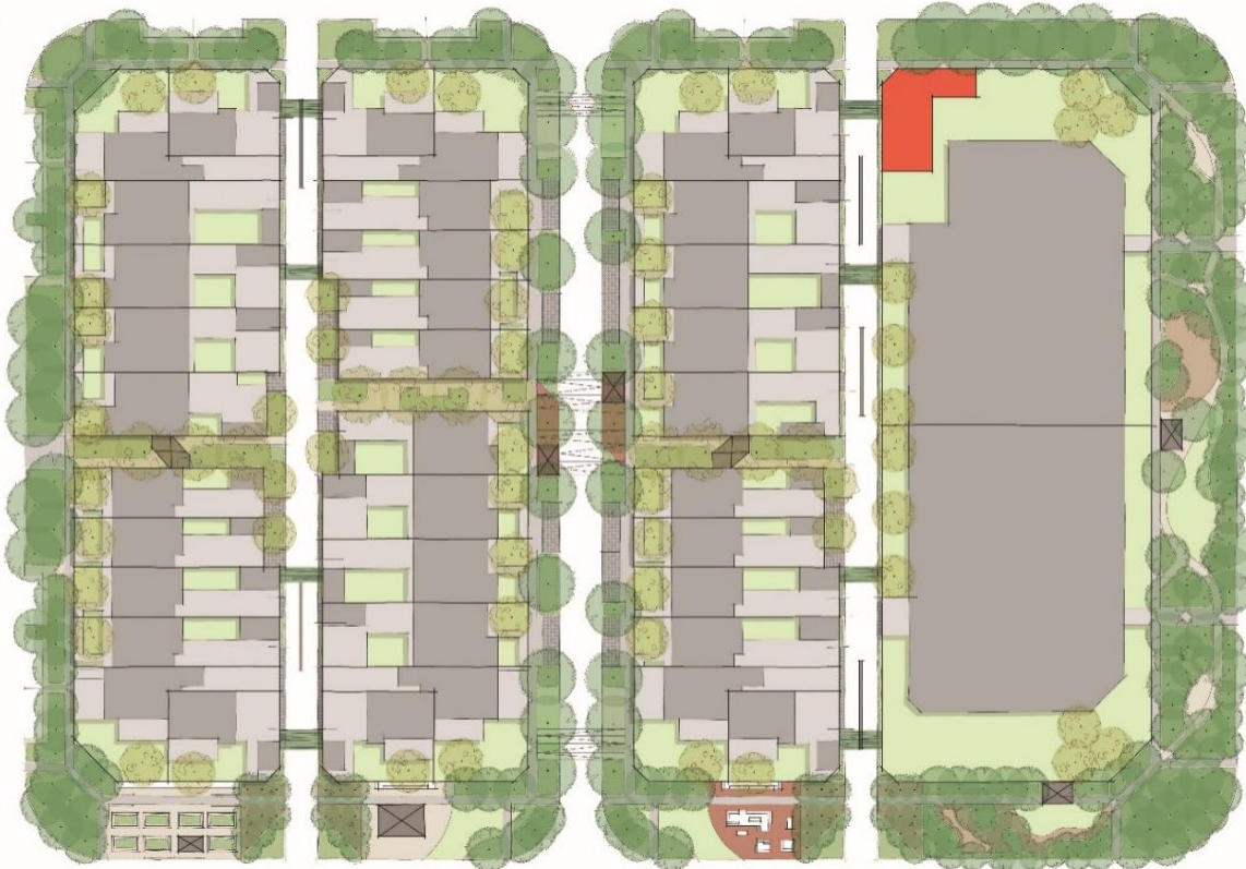
Figure 3 East Village - Knutsford - illustrating the 36 strata dwellings and the two apartment lots to the east of the site and the area depicted red is the precinct battery (Source: LandCorp/ JBA)
