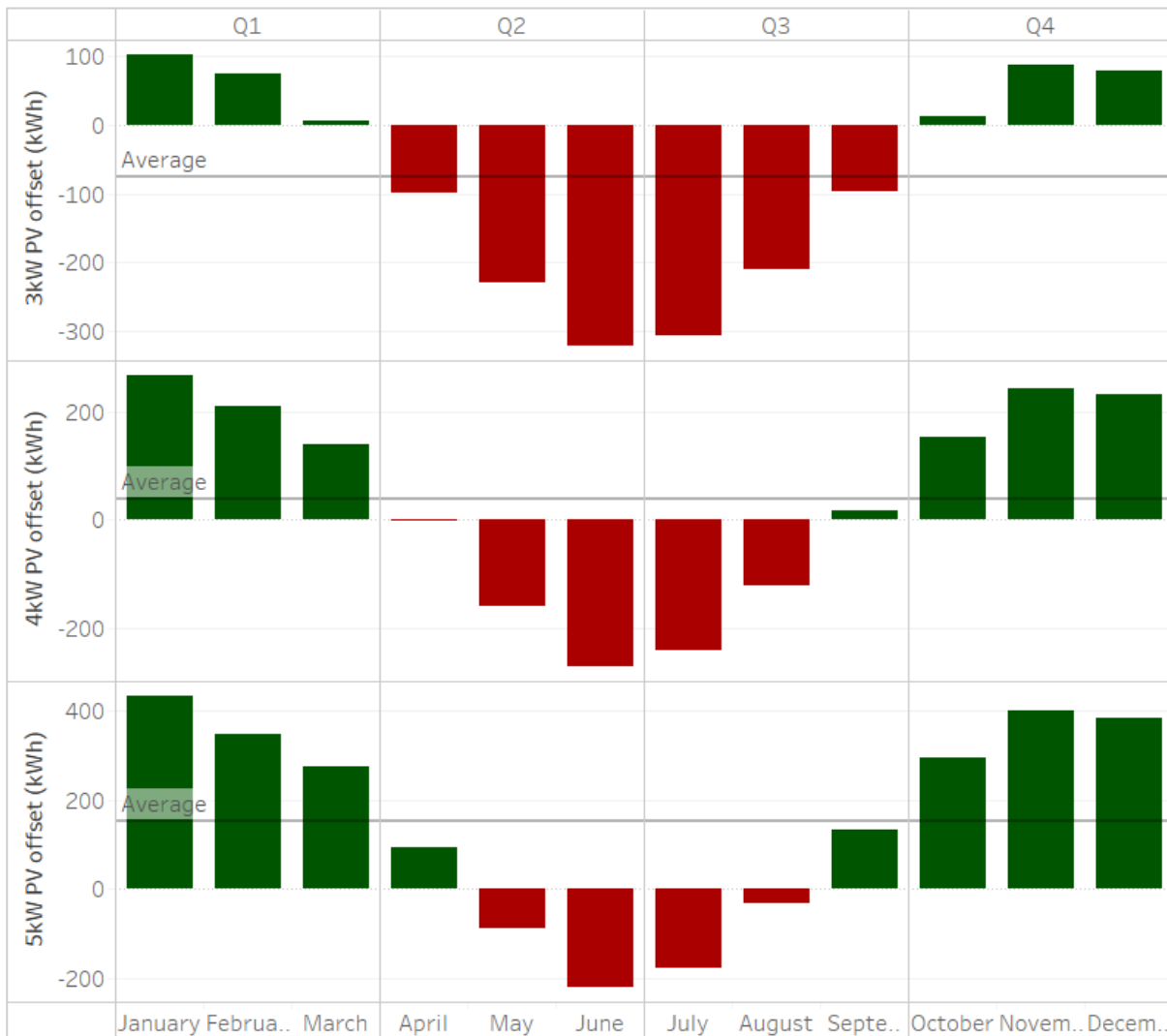
Figure 4 3 kW, 4 kW and 5 kW PV offsets assuming a typical occupancy scenario.
