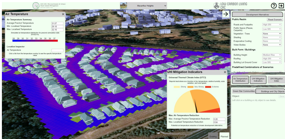
Figure 17: Example of part of planned dwellings in Macarthur Heights and overlay of potential ground cover surface temperature distribution from the UHI-DS Tool
