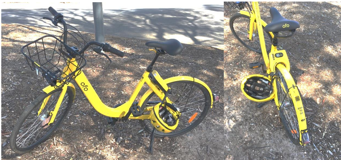
Figure 3-25 a) Parked dockless OfO Bike in Adelaide showing basket and other features; and b) OfO Bike locking mechanism and unique QR Code
