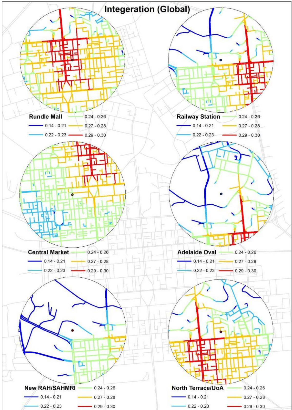
Figure 4- 4 The quality of integration (global) across six major destinations (vicinity of 800 metres)
