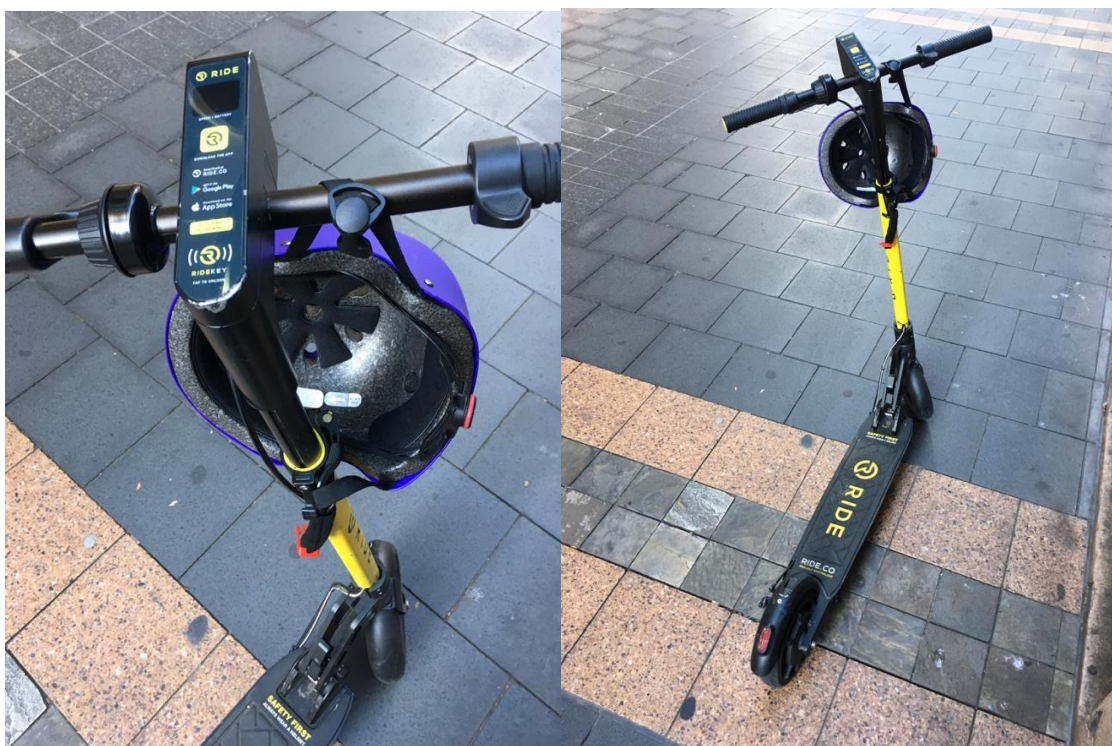
Figure 3- 27 a) Rival Australian Melbourne e-scooter 'Ride' showing height adjustable handle bars, bell, throttle and brake controls, rider instructions and b) E-scooter in parked position with footstand under footplate activated.
