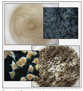
Figure 1: Comparison of conventional activated sludge flocs (top) to aerobic granular sludge microbial granules (bottom); 10x magnification.
