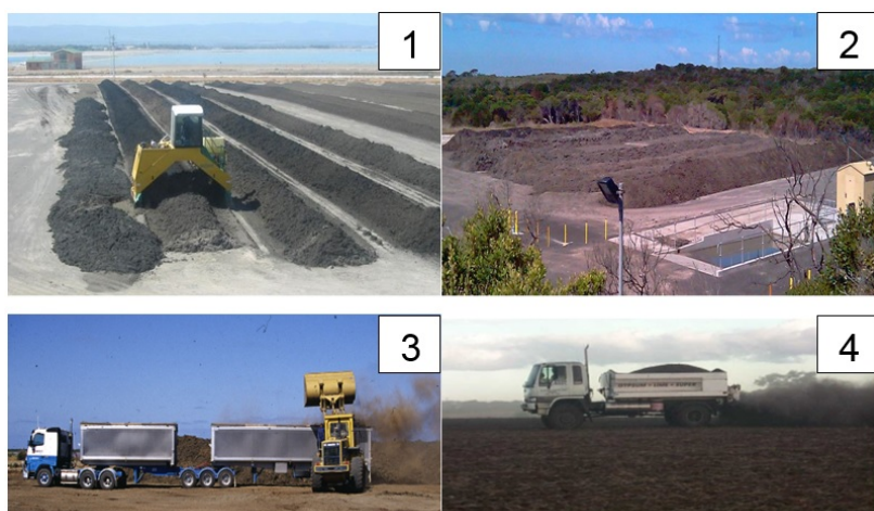
Figure 1. [1] Agitated air drying (AAD); [2] Biosolids hardstand; [3] Loading biosolids into farmers' trucks; [4] Application of biosolids via gypsum spreader
