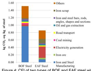
Figure 4: CFI of two types of BOF and EAF steel with the use of iron and steel scrap investigated
