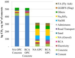
Figure 3: CFI of two types of concrete investigated with either NA or a 100% replacement with RCA
