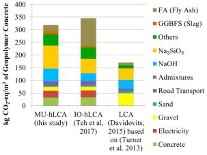
Figure 2: Contributions of main GHGEs for the production of GPC by MU-hLCA, IO-hLCA and LCA
