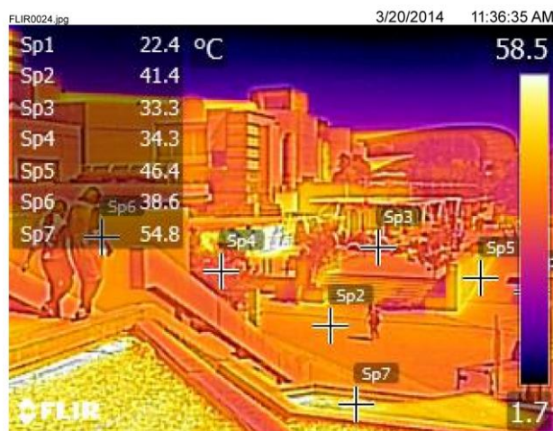
Figure 1: Some hard urban surfaces such as asphalt, concrete and paving store heat in their thermal mass and make the public space a dangerous place to attend during heatwaves (Riverbank Plaza, Adelaide, FLIR 6 thermal image taken by E. Sharifi).
