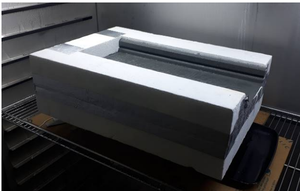
Figure 10: Steel roof sheet sample fitted to the polystyrene enclosure, within the climate chamber.
