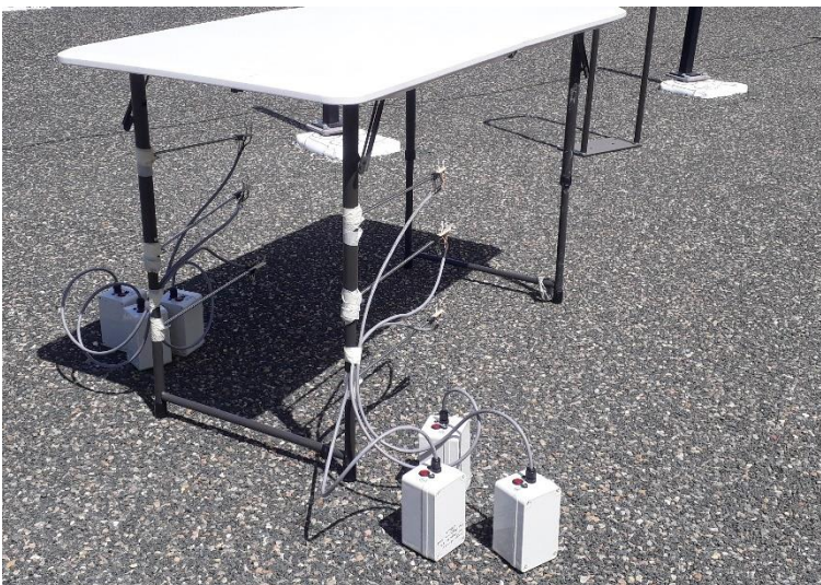
Figure 3.9: Test to investigate the sensitivity of Modern Device rev. P wind sensors to direct solar radiation.
