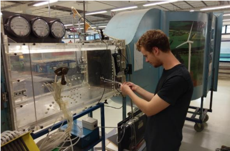
Figure 3.8: Wind tunnel calibration of the wind speed sensors.
