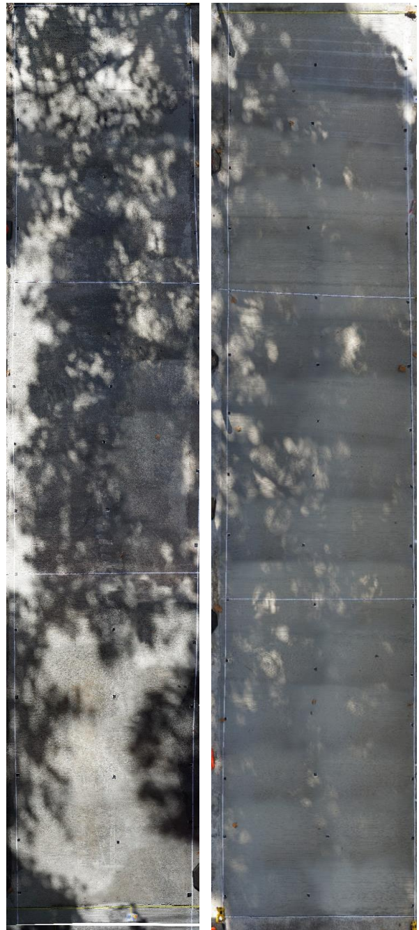
Figure 12. High resolution photogrammetry of (a) GPC and (b) OPC concrete pavement slabs.
