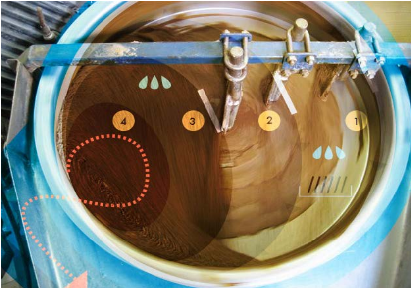
Figure 7: A diagram overlaid on this actual running palletiser shows how the principles apply to the real-life operation of a palletiser.
