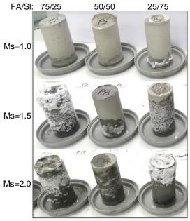
Figure 3: Effect of the precursor's proportion, and different modulus ratios on the efflorescence of geopolymer pastes, (one month exposure to water)
