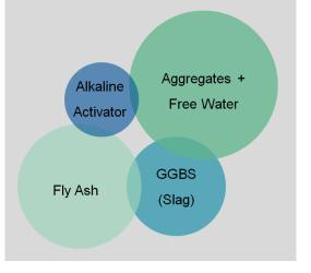
Figure 1: Geopolymer concrete constituents
