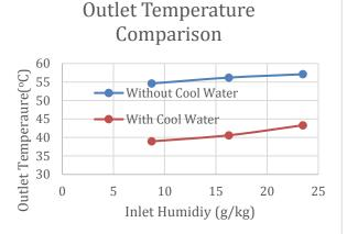
Figure 3: Outlet temperature comparison between conventional wheel and internal cool wheel
