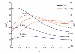
Figure 4: Coefficient of performance (both electricity and thermal) for new air-conditioning system.
