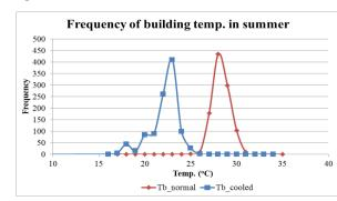
Figure 5: Frequency of base building temperature in summer (hourly, 1 degree bins).
