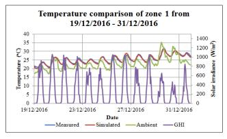
Figure 3: Measured and simulated temperature comparison.
