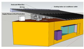
Figure 1: Final design of the PV/T desiccant wheel cooling system
