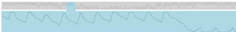
Figure 9 Stored energy profile for a year, for Household 1 with 5 kWh of usable energy storage. The top portion of the graph shows the stored energy profile for the entire 2013 year; the lower portion, with the blue background, shows detail from a two-week period. The vertical axis on each subgraph is stored energy, from 0 to 5 kWh.
