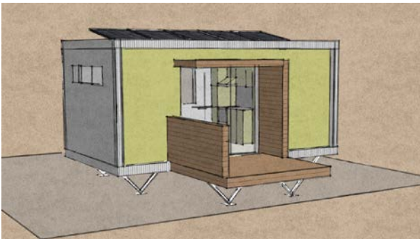
Figure 39 - Perspective of the front of the Pod with metal cladding and painted FC in the north wall
