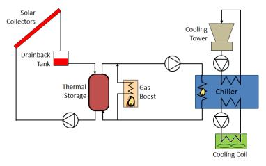
Additionally, experiments will be conducted at CSIRO to determine the feasibility of next generation solar absorption cooling systems.
