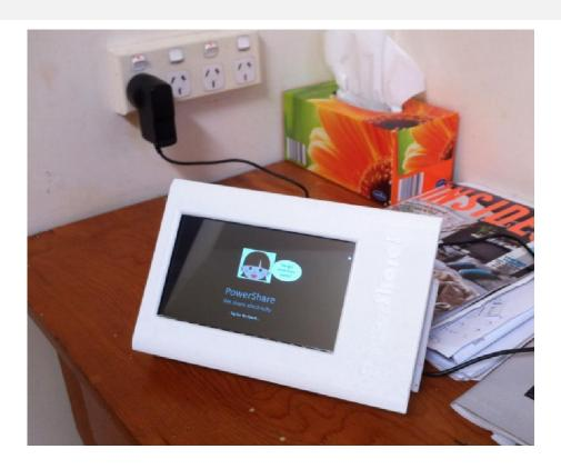
Figure 2: The in-home display is connected to the smart meter as well as data sources such as the Bureau of Meteorology, PVWatts.org and other IHDs
