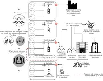
Figure 4 Australian electricity sector with SPMs. (a) Centralised large scale power plants owned by private companies connected to large industries through the transmission network; (b) energy retailers or other intermediaries; (c) alternative energy providers; (d) stand-alone system or prosumer to micro-grid. Taking electricity as starting point, Figure 4 shows the Australian electricity sector represented with SPMs, as an example of the concept's applicability, modularity and flexibility.
