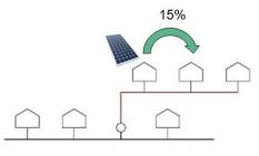
Figure 2. Schematic diagram of an embedded network. The top three houses are on an embedded network. The circle represents the common connection point to the public distribution network.
