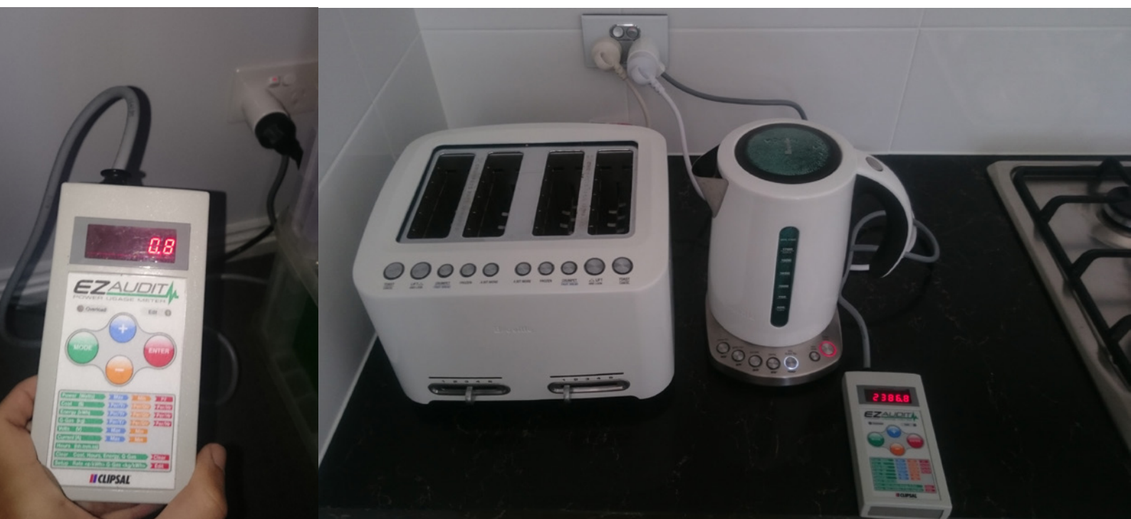
Figure 2.2 A power meter measuring the standby power drawn by a smart power board (0.8W) and a smart kettle (2.39kW). Source: DM Whaley
