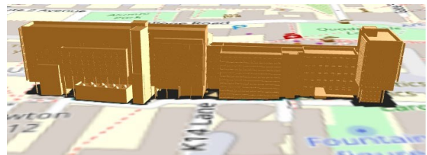
Figure 19 The 3D georeferenced Red Centre model visualised on QGIS (with the DTM values used as height for the terrain)
