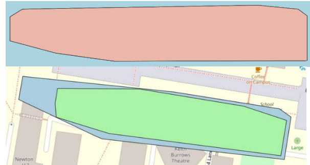
Figure 15 (Top) BIM geometries reprojected on the Pseudo-Mercator map. (Middle) Its corresponding convex hull. (Bottom) Convex hull of the EM footprints (green) and the one of the OSM building layout (blue)
