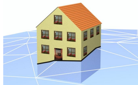
Figure 1. TerrainIntersectionCurves in CityGML (Gröger et al., 2008).
