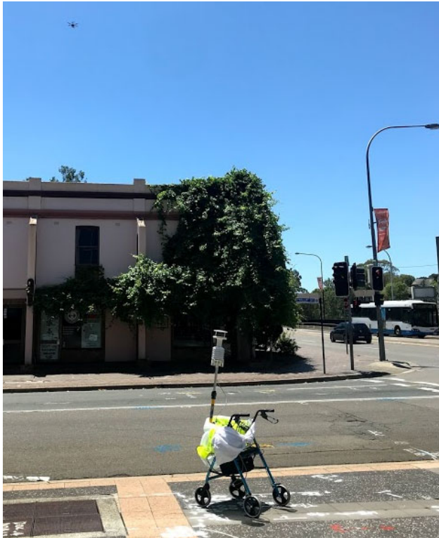
Figure 8. The MetPak Pro weather station in Phillip St. mounted on a cart at 1.5 m from the ground and the flying drone in the sky.
