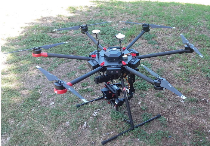
Figure 6. The drone and thermal camera of the HPA group of UNSW Built Environment used for the thermal survey.
