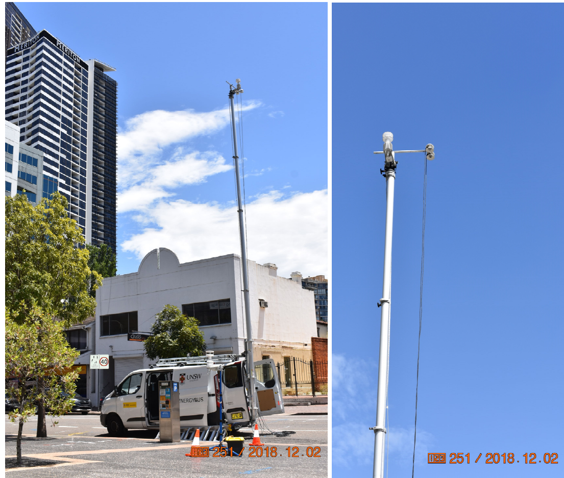
Figure 1. The EnergyBus in Phillip St. with the monitoring station mounted on the mast at 10 m from the ground.
