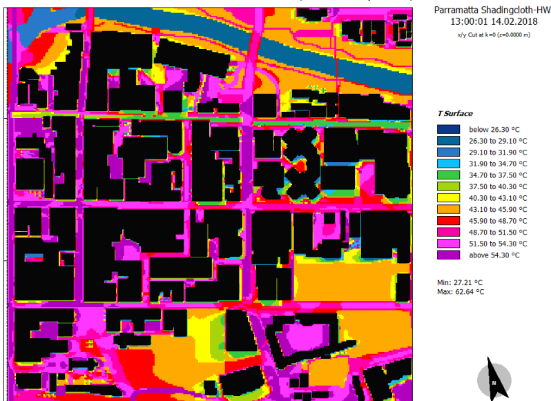
Figure 108. Distribution of surface temperature in the City of Parramatta CBD and Phillip St: Scenario 3, heatwave condition - 13:00
