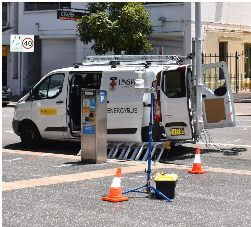
Figure 2. The MetPak Pro weather station in Phillip St. mounted on a tripod at 1.5 m from the ground.
