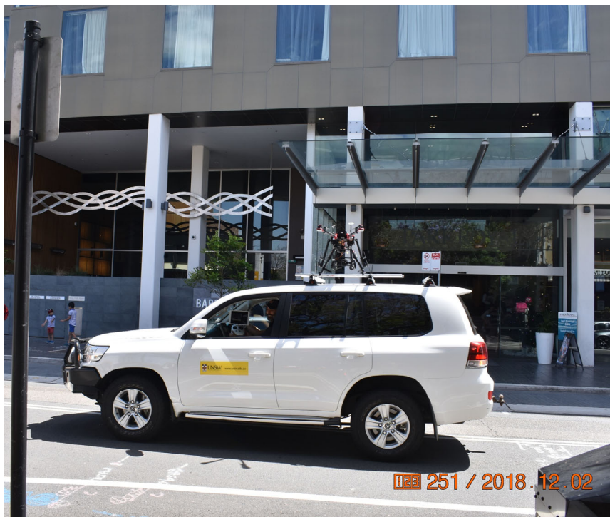
Figure 5. A car used for the terrestrial survey, equipped with the UNSW drone.
