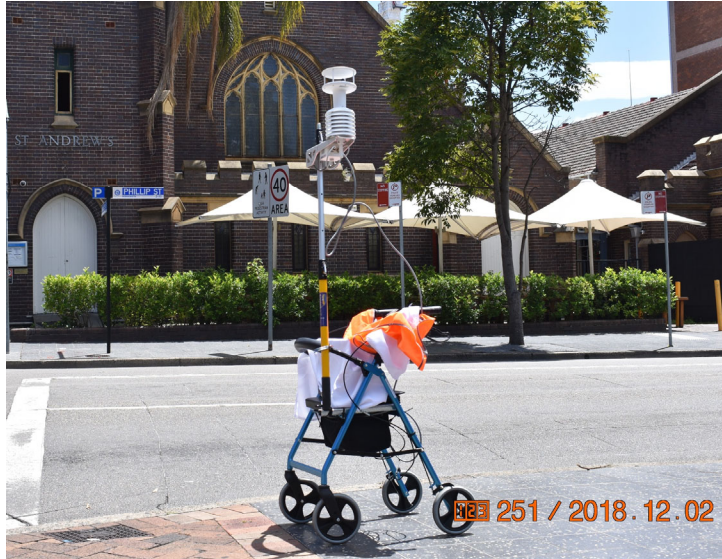
Figure 3. The MetPak Pro weather station in Phillip St. mounted on a cart at 1.5 m from the ground used for spot measurements in Track M.
