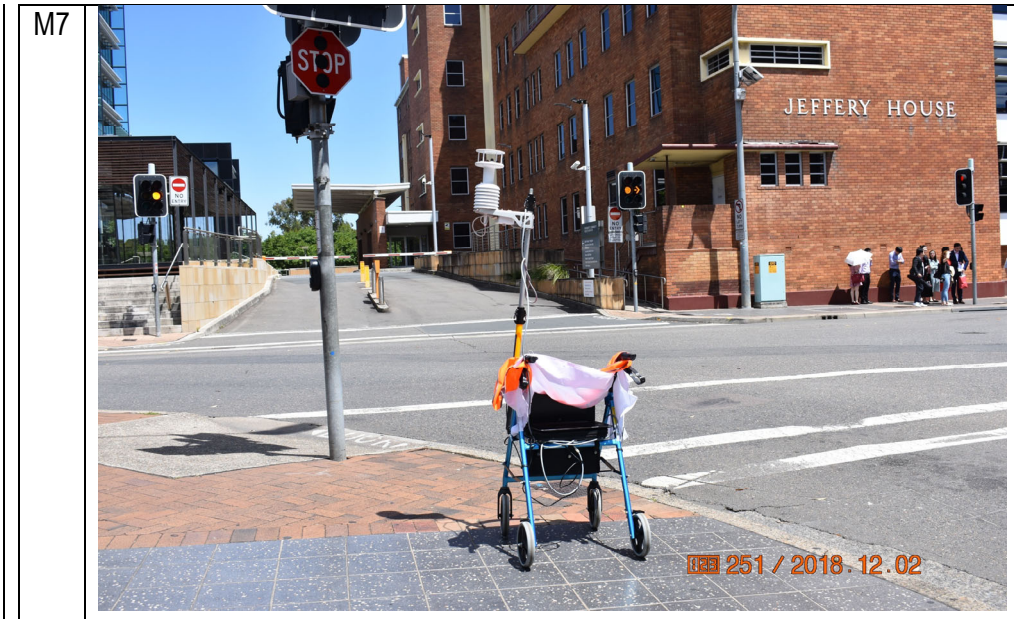
Figure 10. MetPak Pro weather station on the cart at each measurement locations of Track M.
