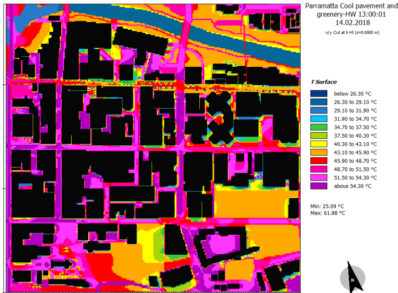
Figure 128. Distribution of surface temperature in the City of Parramatta CBD and Phillip St: Scenario 7, heatwave condition - 13:00
