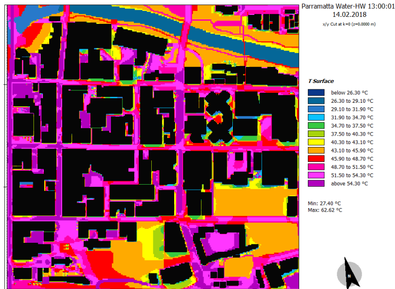
Figure 113. Distribution of surface temperature in the City of Parramatta CBD and Phillip St: Scenario 4, heatwave condition - 13:00
