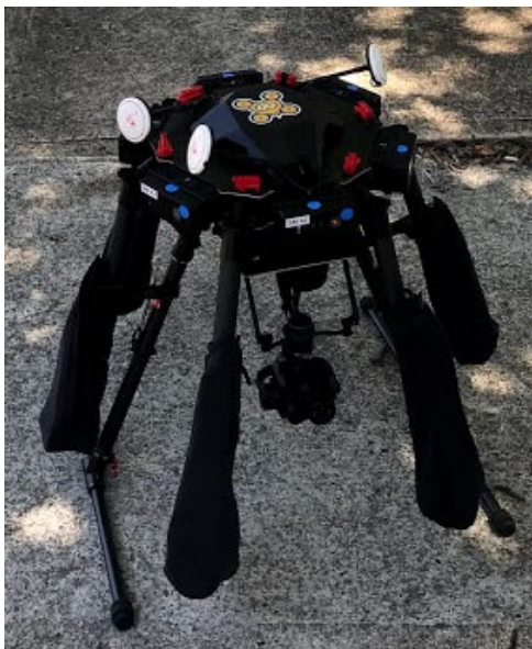
Figure 7. The drone and thermal camera of SkyMonkey used for the aerial survey.
