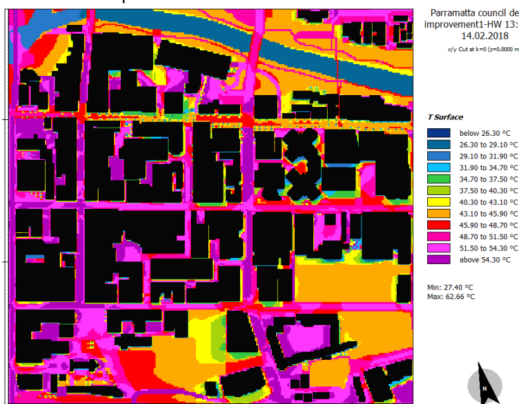
Figure 143. Distribution of surface temperature in the City of Parramatta CBD and Phillip St: Scenario 10, heatwave condition - 13:00
