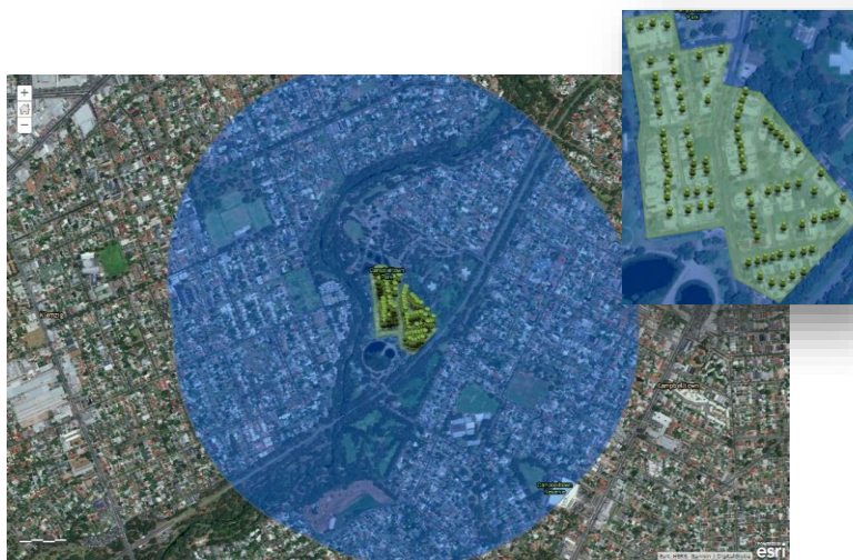
Figure 6. The information and data collection area for model inputs expands in an 800m buffer beyond the centroid of any land-parcel contained within the precinct under analysis.
