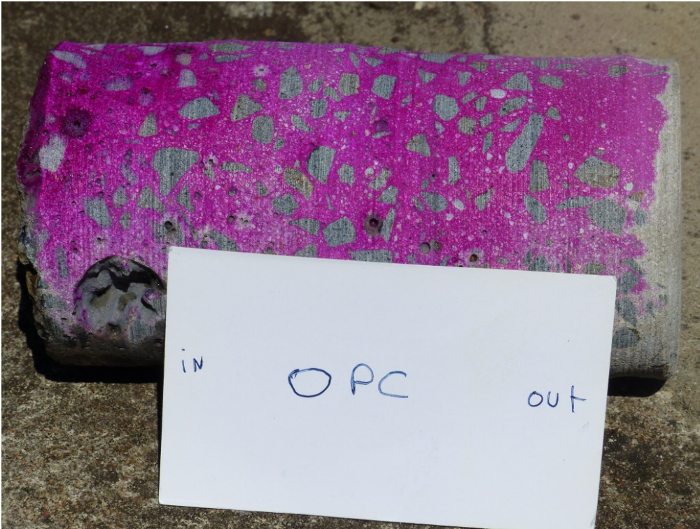
Figure 17. OPC Concrete core from water tanks at Toowoomba site, QLD, in December 2015.
