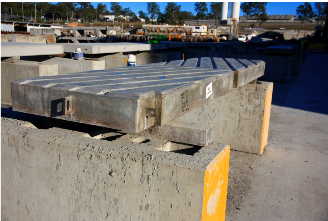
Figure 102. Completed EFC boat ramp plank after curing.
