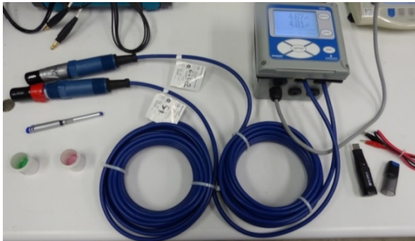
Figure 109. pH probe and data transmitter system.
