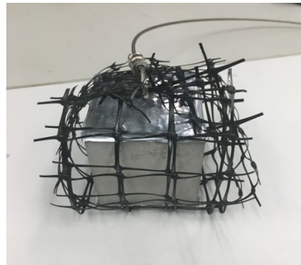
(b) After placing the specimen inside the net for hanging.
