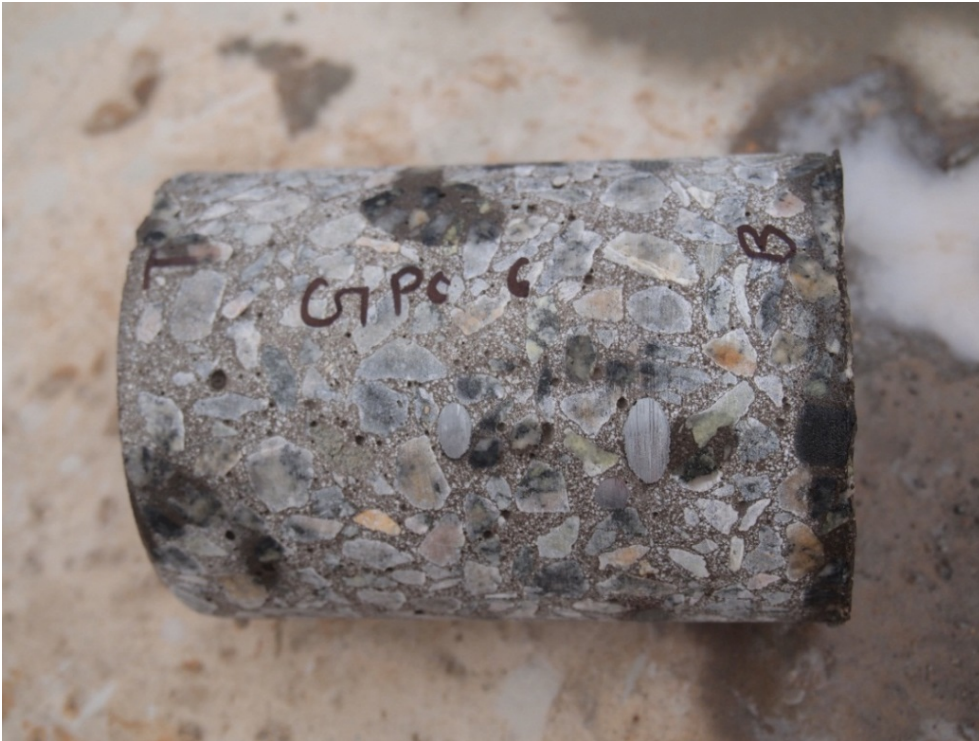
Figure 24. Typical Geopolymer concrete core sample from Lake King site, WA, in October 2015.
