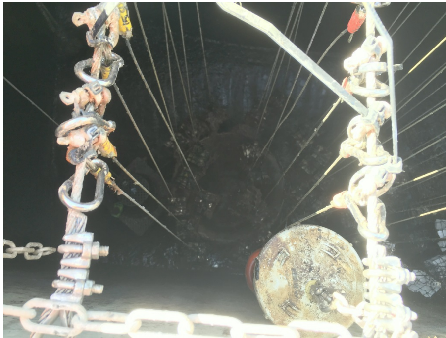
Figure 124. Specimens at the time of removal from digesters.
