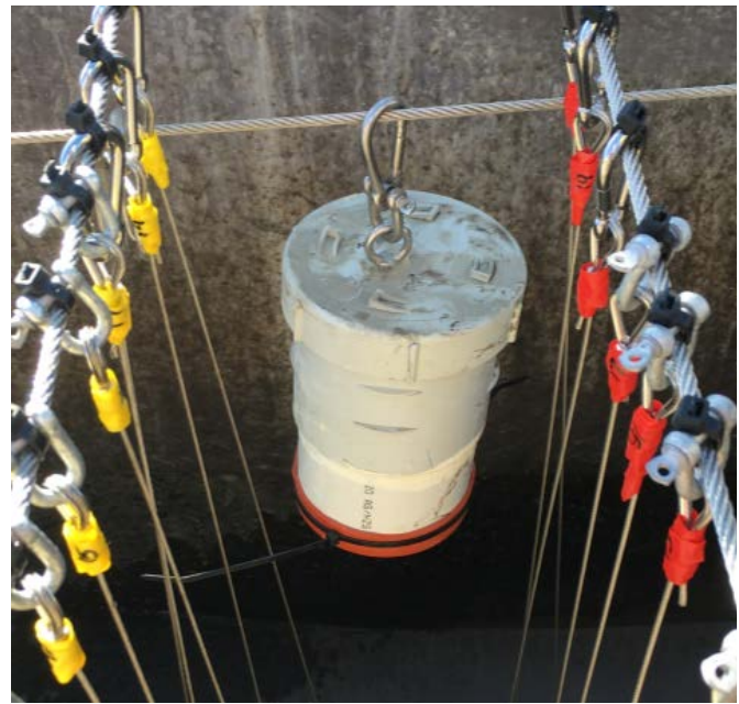
(b) Placed inside drain hanging from wire.
