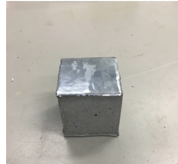
(b) Specimen with sealed top and bottom.
