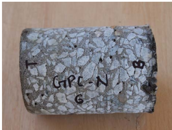
Figure 45. Typical Geopolymer concrete core from culvert at casting yard in Perth, WA, in October 2015.
