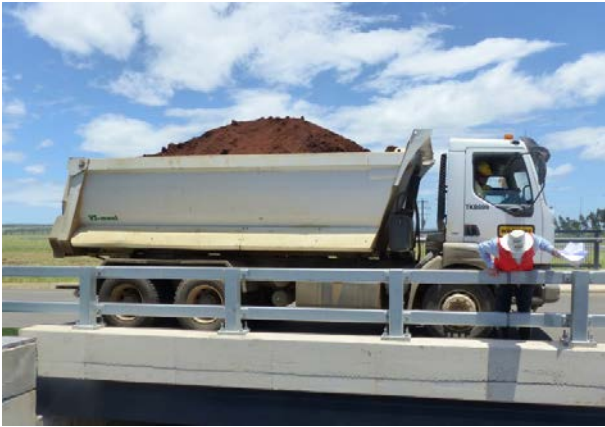
Figure 78. Live load testing: truck position 1.
