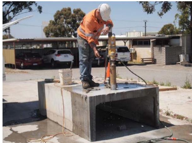
Figure 44. Coring of OPC concrete culvert at casting yard in Perth, WA, in October 2015.
