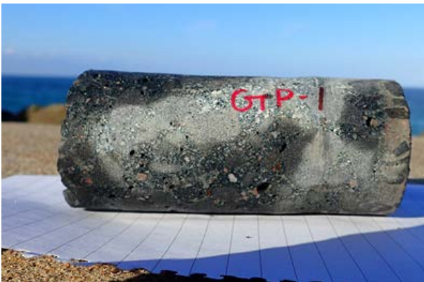
Figure 56. Typical Geopolymer concrete core from block at Portland, Victoria, in June 2016.
