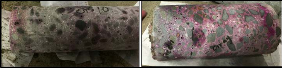
Figure 6. No clear carbonation front by phenolphthalein indicator for Type 1 and Type 2 specimens
