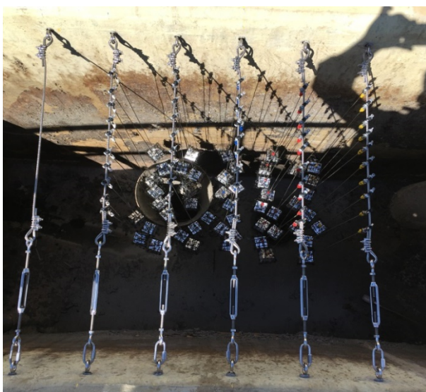
Figure 121. Specimens hanging pattern in each digester.
