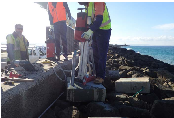
Figure 55. Coring of GPC block at Portland, Victoria, in June 2016.
