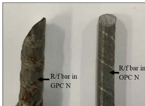
Figure 50. Visual observation of embedded steel bars extracted from GPC and OPC concrete at 8 years exposure (45 mm cover).
