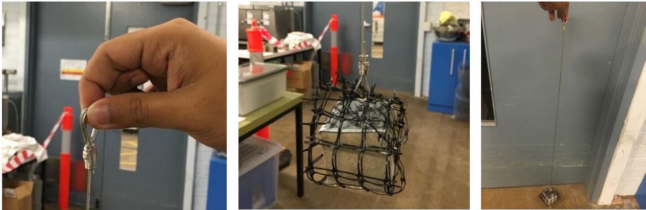
(a) Top swage for attachment to connecting line. (b) Bottom swage connection to net basket. (c) Specimen hanging.
