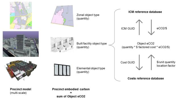
Figure 1 Calculating embodied carbon using ICM metrics
