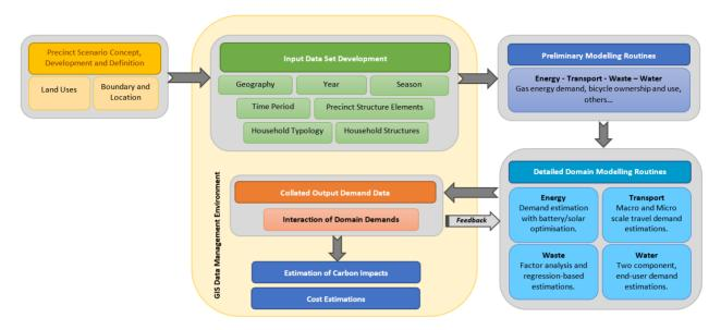
Figure 2 ETWW operational flowchart
