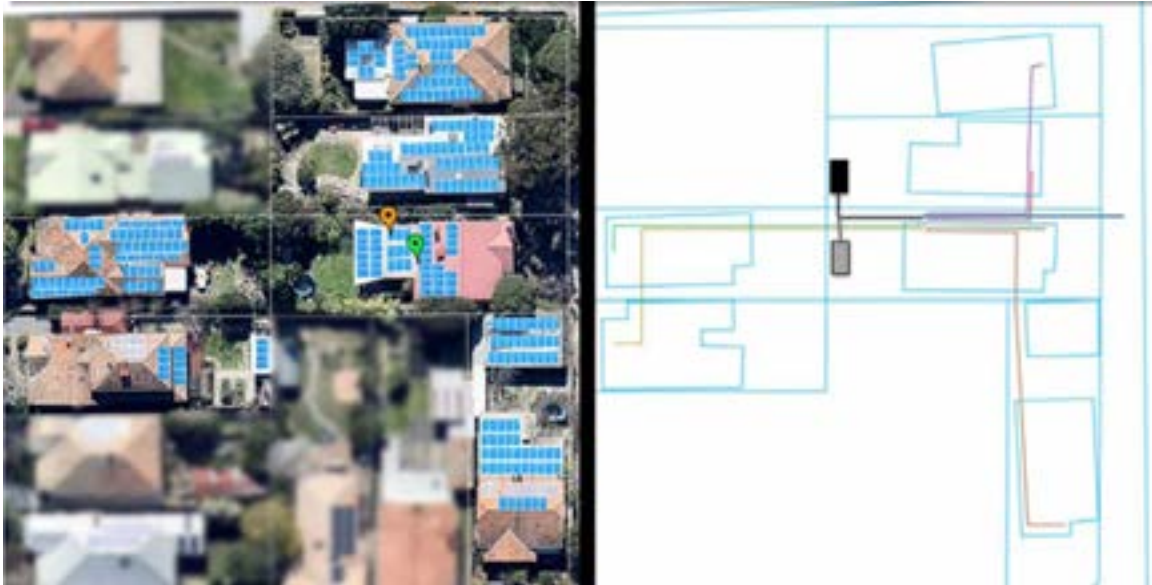
Figure 1. A modified image showing a group owned solar system at left, and potential local network with central battery storage to distribute and share generated electricity at right.
