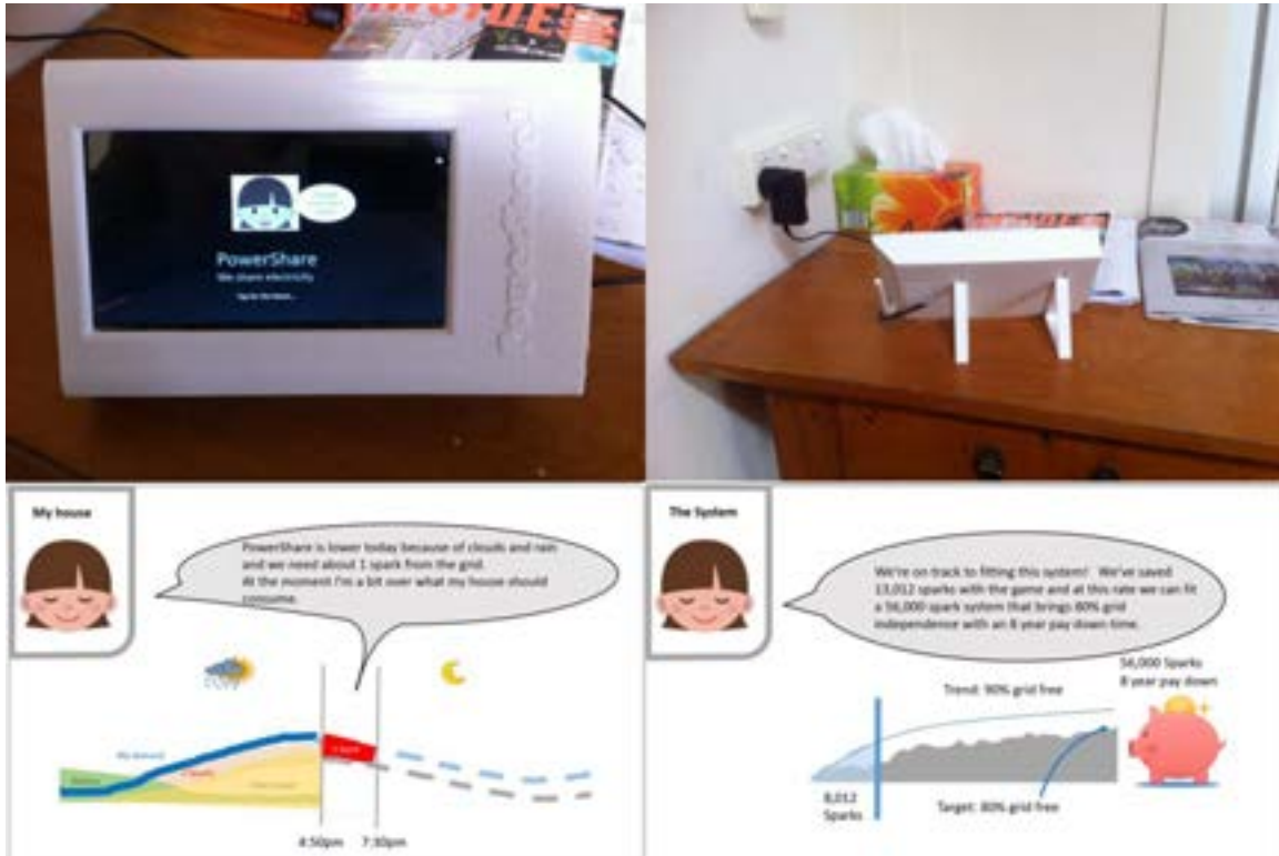
Figure 2. Top left: experiment in-home energy display. Top right: in-home energy display rear view with LoRA radio antenna visible. Bottom left: Performance, generation and goal for participant home. Bottom right: final goal for the group. The display communicates with the home smart meter and with a central server via an internal 3G dongle. The IHD does not interact with conventional electricity billing at all.
