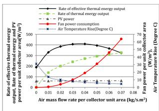
We have modelled the above mentioned BIPV/T air system in TRNSYS. The results of the simulation were compared against the experimental data from the house. Figure 4 shows that there is a good agreement between simulated data and measured data.
