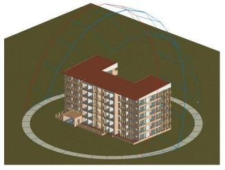
Figure 2: 3D model of case study multi-storey residential prefabricated building, for the Thermal Performance simulation.
