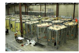
Figure 3: Industrialisation of the fabrication of bathroom pods
